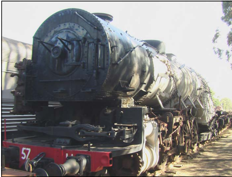
The once mighty 3-cylinder 5711 waits up at the southern end of the RTM part way through a static restoration. Much of the locomotive is overshadowed by its massive boiler and smokebox. February 17, 2007.
